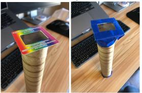
2. On the other end of the tube, place two pieces of tape parallel to each other forming a slit in the middle.
