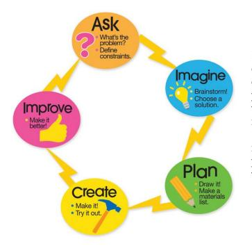
Engineers work together through the engineering design process. It is a cycle that not only helps scientists create a solution to a problem, but helps them work through testing their product and making improvements as necessary. It sometimes takes hundreds of "redo's", or making improvements and re-testing, before a product is ready for the public. Rarely do scientists get it exactly right on the very first try! So, don't give up!
